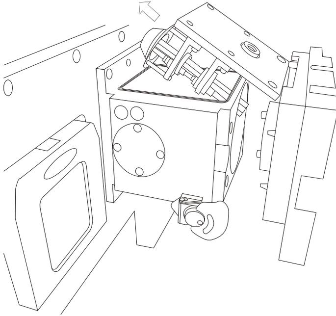
11. Remove the hexapole from the assembly by loosening the four captive screws, separating the three cable splitters and then detaching the hexapole from the base plate.
