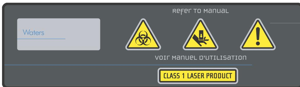
When you follow the operating procedures described in this manual, the laser beam remains contained within the instrument, and no risk of personal exposure to laser radiation ensues.
