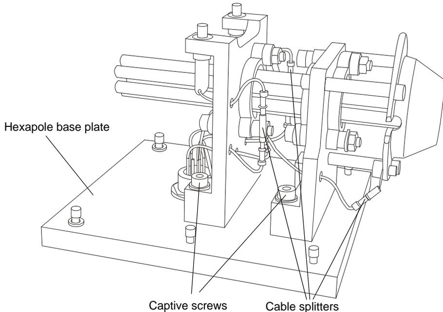
12. Wash the hexapole using a wash bottle filled with propan-2-ol (IPA).
