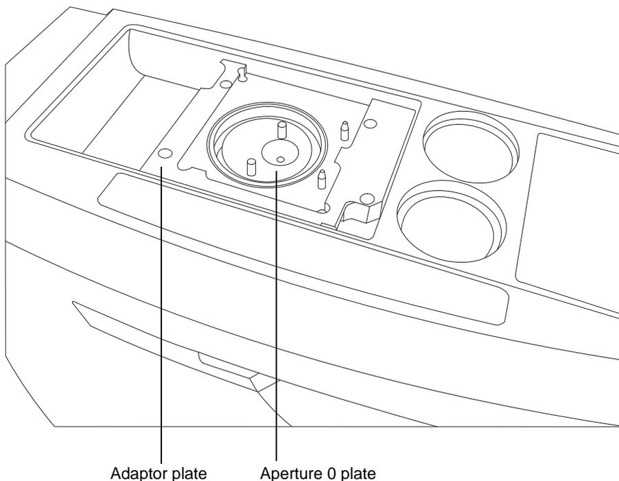
6. Locate the adaptor plate and aperture 0 plate, which are stored in the rectangular recess inside the component repository.
