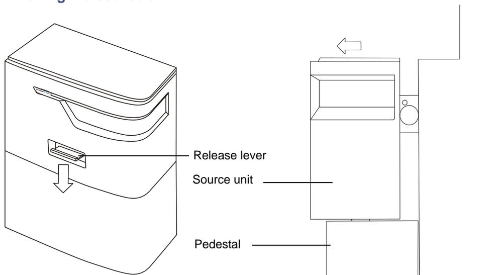
10. Press and hold the Raise button until the source unit fully extends above the pedestal.
