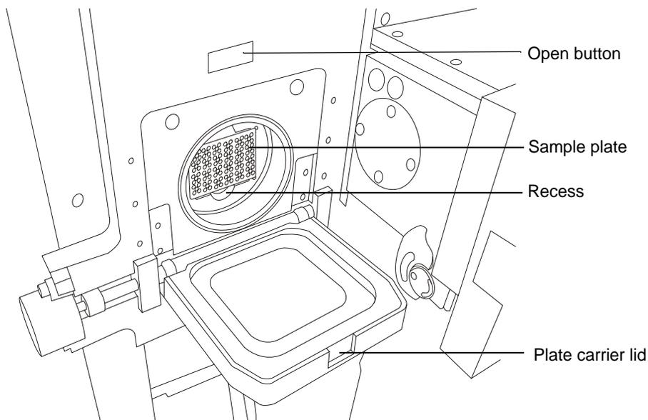
2. Hold the sample plate by the sides, orienting it so that the corner indentation faces the bottom left-hand side, and then place the plate into the recess within the plate carrier.
