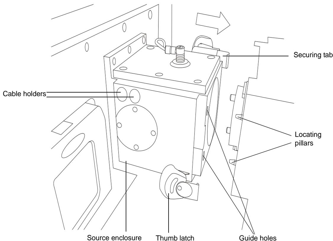
13. Release the two securing tabs on either side of the source enclosure by pulling the thumb latches towards you and rotating them counterclockwise.
