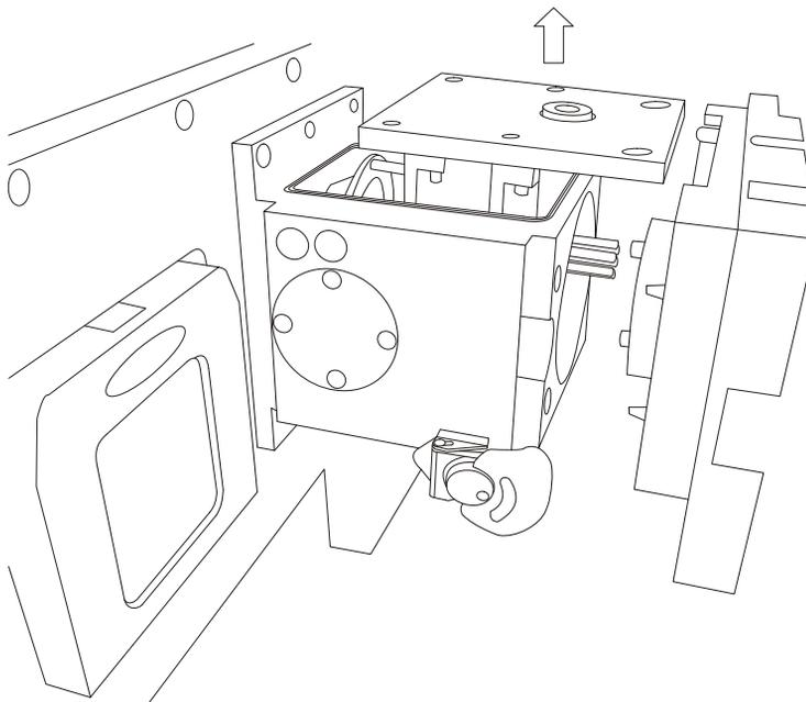
10. Tilt the hexapole assembly by approximately 45°, and then withdraw it carefully from the source housing.
