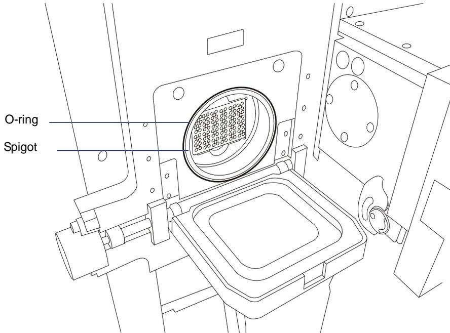
3. Clean the O-ring and its seating surface with a lint-free cloth and methanol.
