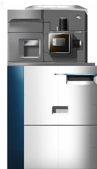
The image shows a MALDI SYNAPT G2 HDMS system with a LockSpray™ source fitted.
